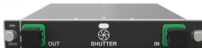
With or without the power monitoring option, the FTBx-3500 module occupies just a single slot.
