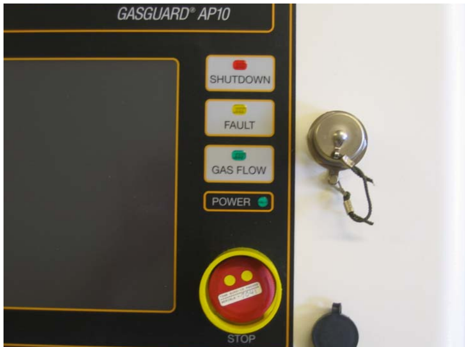
Figure 4.10: AP10 Controller with USB Port Capped
