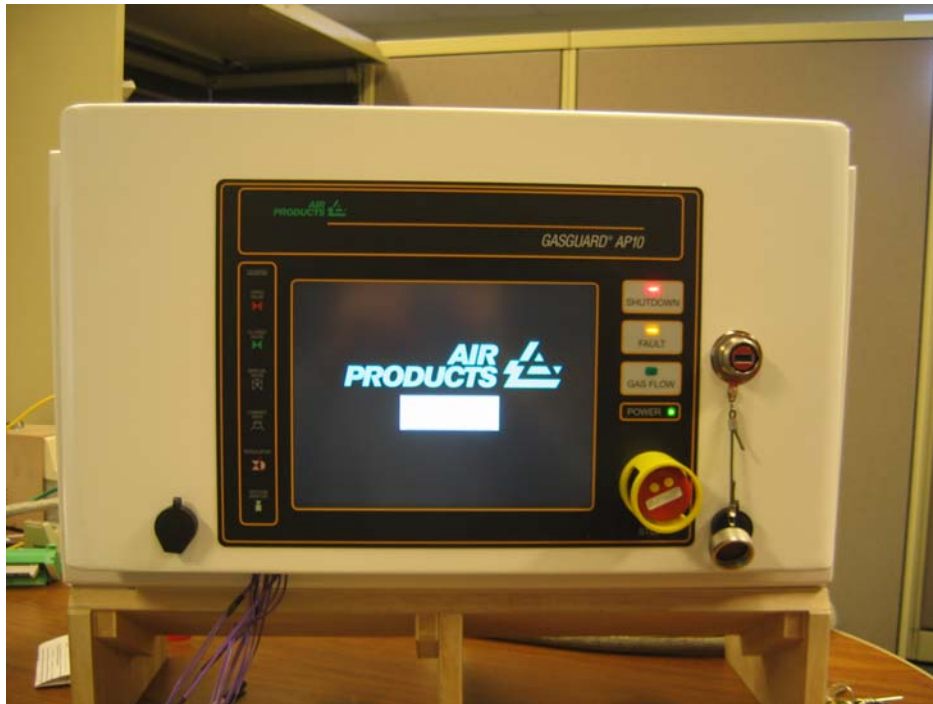
Figure 4.9: AP10 Controller with USB Port on the Face of the Controller
