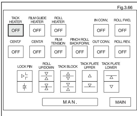
On the manual screen of the operation panel, press the TACK HEATER "OFF" button to turn it "ON."
