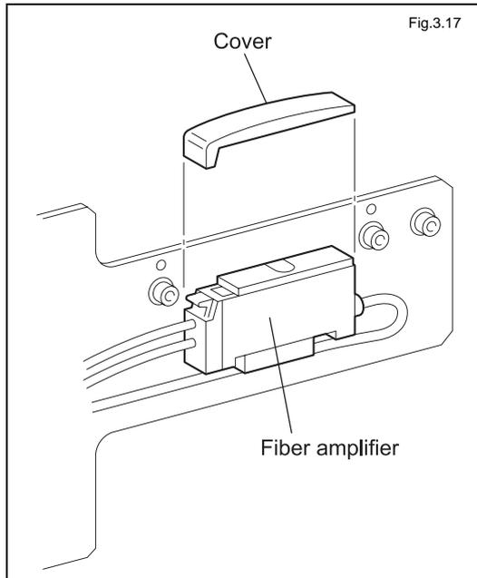
Remove the cover of the fiber amplifier.
