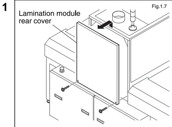
Remove the lamination module rear cover.
