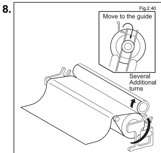
Fix the cover film to the eco-roll by running it under the dry film, and transfer the eco-roll from the holding bracket to the guide section.
