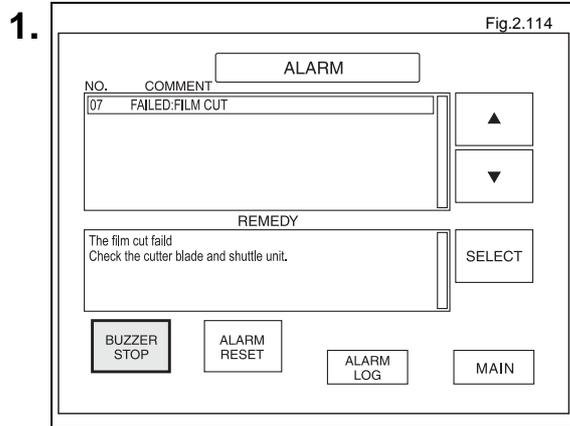
Press the "BUZZER STOP" button on the alarm screen to stop the buzzer.
