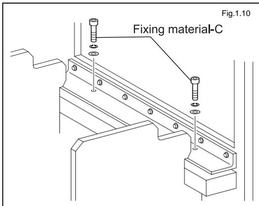
Remove fixing material C.
