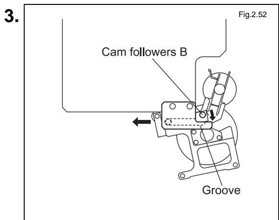
Slide cam followers A to the end of the groove, and lower cam followers B to the groove in order to fix the lower DF unit to the attachment.
