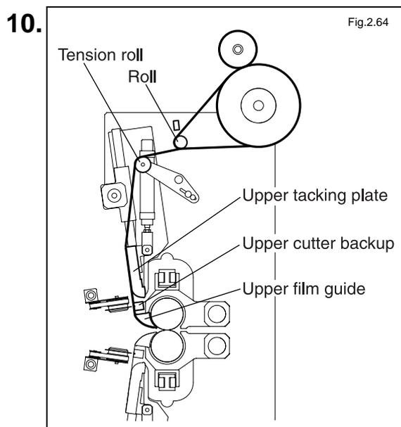
Run the laminate film along the film-running surface as shown in the illustration to the left.
