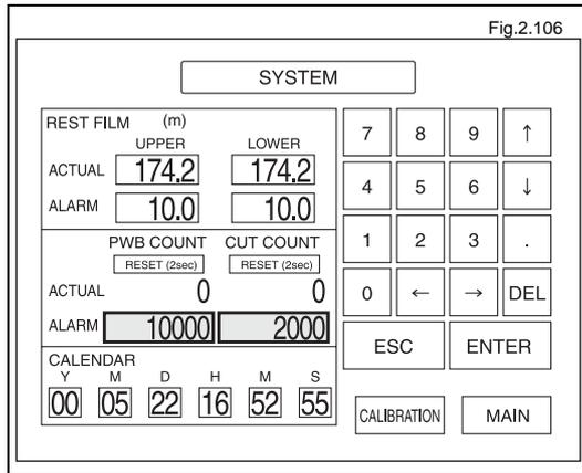
Press the square frame of the "ALARM" values of the PWB COUNT and CUT COUNT.
