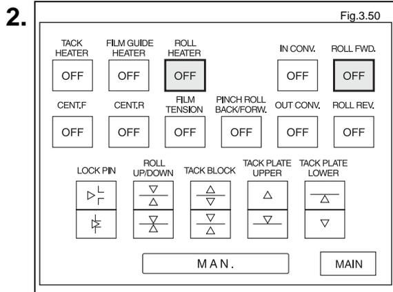
On the manual screen of the operation panel, press the ROLL HEATER "OFF" button and the ROLL FWD "OFF" button to turn them "ON" and rotate the laminating roll forward.
