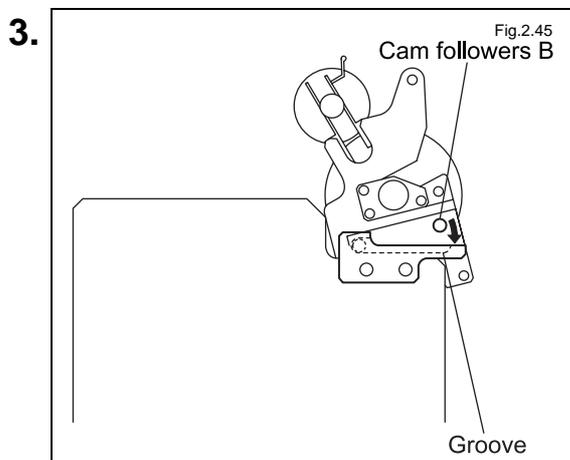
Slide cam followers A to the end of the groove, and lower cam follower B to fix the upper DF unit in the groove of the attachment.
