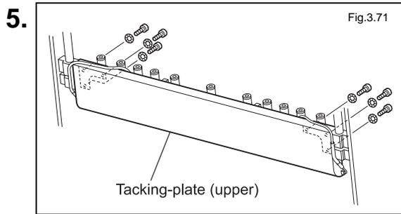
Remove the tacking-plate fixing screws.
