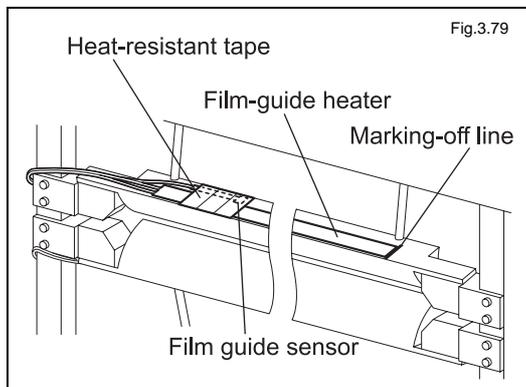
Stand in front of the lamination module. Peel off the heat-resistant tape and remove the film-guide heater.
