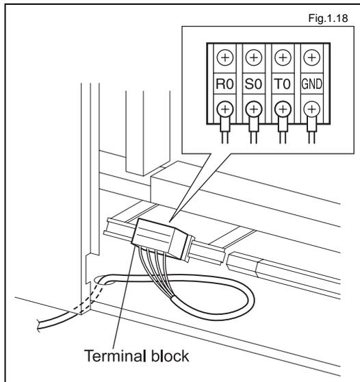
Confirm that power cables are laid through the inlet at the bottom of the control box at the rear of the unit from the power source of the plant, and that they are connected to the unit.
