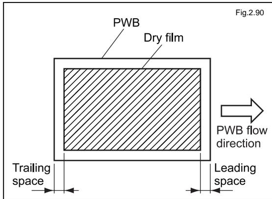
Follow the steps specified below to set the spaces on the leading and trailing edge of the board where the film will not be laminated onto the PWB (length in mm.)
