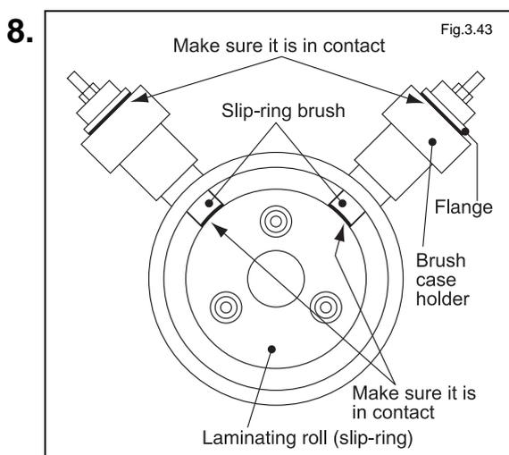
Fix the slip-ring brush and visually inspect the contact condition.
