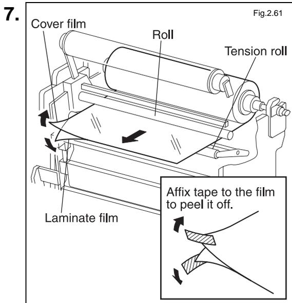
Pull out the dry film, run it between the roll and the tension roll to separate the laminate film from the cover film.
