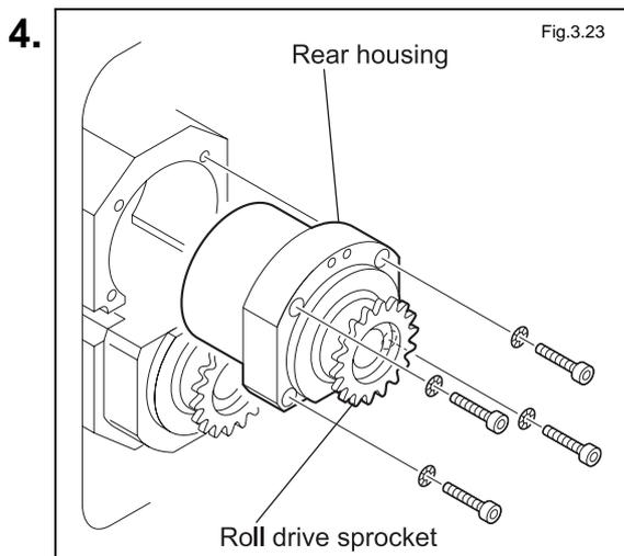
Remove the rear housing together with the roll drive sprocket.
