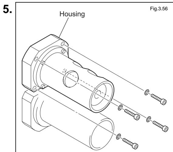
Remove the cap bolts that hold the housing in place.
