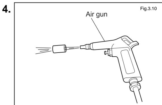
Use an air gun to blow air inside the leak line filter in order to remove dust from the filter.
