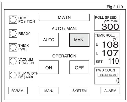
To set to in the manual-operation mode, press the yellow "MAN." button on the main screen.
