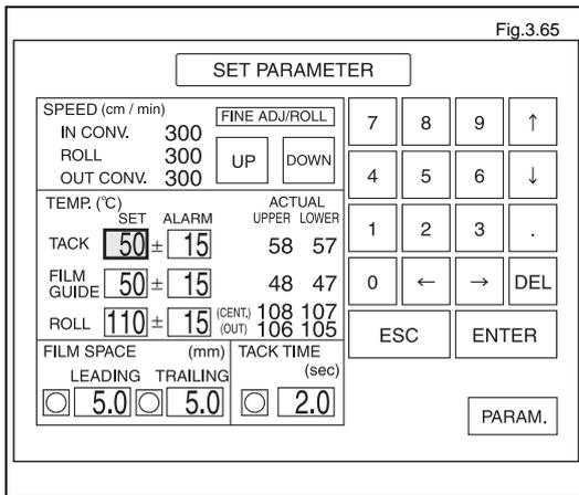
On the parameter setting screen of the operation panel, set the tacking rubber temperature at 50°C.
