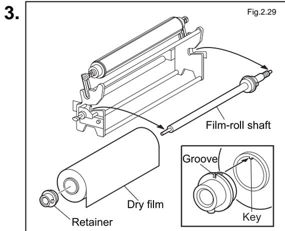
Remove the film-roll shaft from the DF unit and position the dry film at approximately the center of the shaft.
