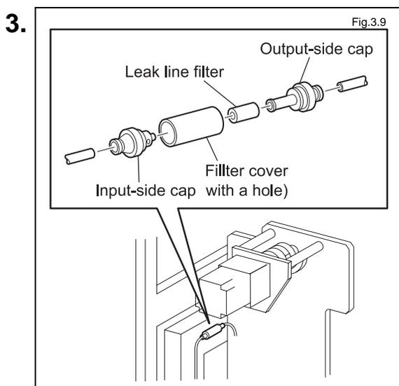
Remove the tube fittings on the output and input sides of the leak-filter assembly, and disassemble the assembly.
