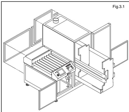
Open the doors and fixed covers of the unit, and wipe away the dirt and dust from the inner and outer surfaces using a clean-room cleaner and a lint-free cloth~ moistened with a neutral detergent.
