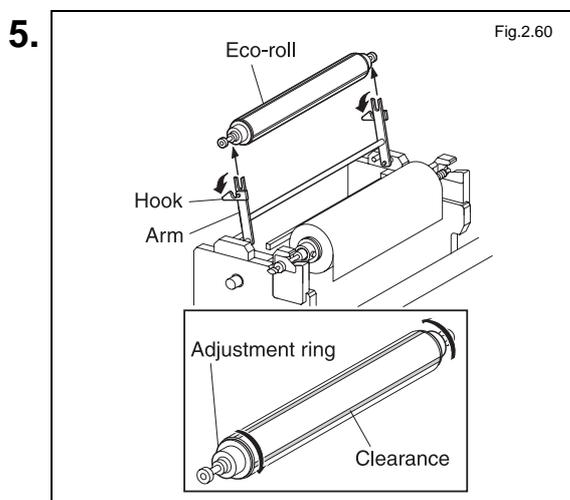
Open the hook to remove the eco-roll from the arm of the upper DF bulk unit, and turn the adjustment ring to make a clearance on the external circumference.
