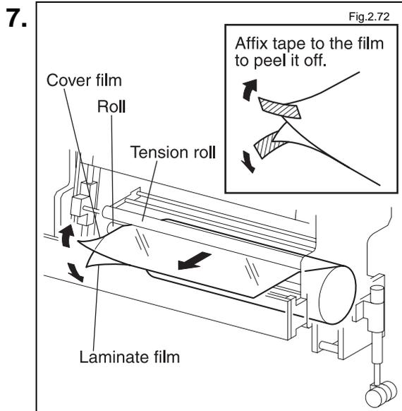
Pull out the dry film, run it between the tension roll and the roll to separate the laminate film from the cover film.
