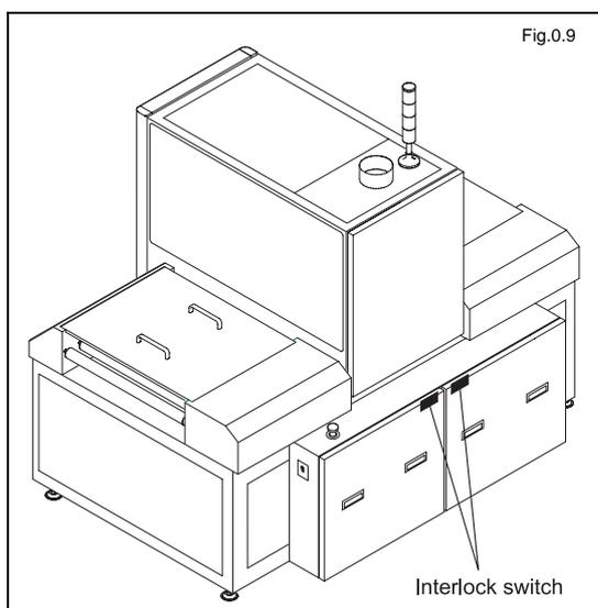
If the control box cover is opened when the unit is in operation, it will immediately stop, as when the operation-panel Power  button is pressed.
