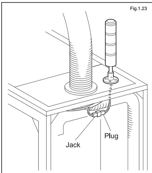
Connect the plug of the signal tower to the jack on the rear of the exhaust duct.
