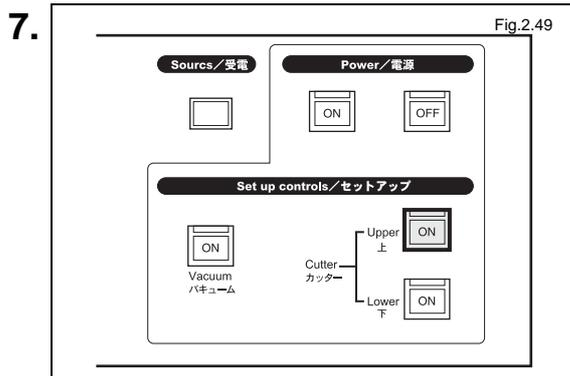
Press the Upper Cutter  button on the operation panel.
