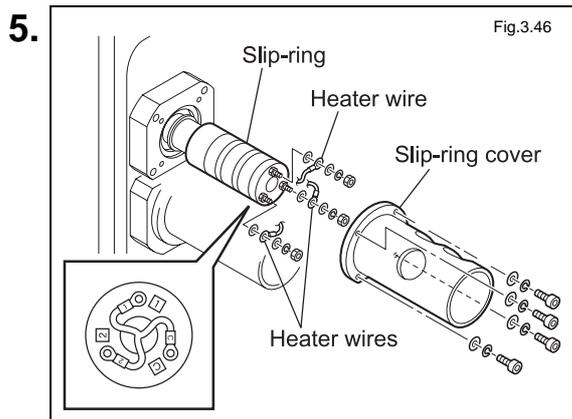
Remove the slip-ring cover and heater cord.
