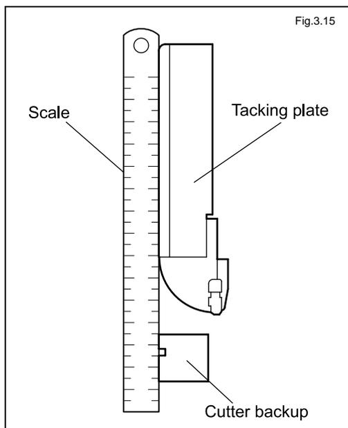
Use a scale to confirm that the tacking plate and cutter backup are flush with each other.
