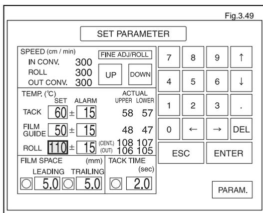
On the parameter setting screen of the operation panel, set the roll temperature at 110°C.
