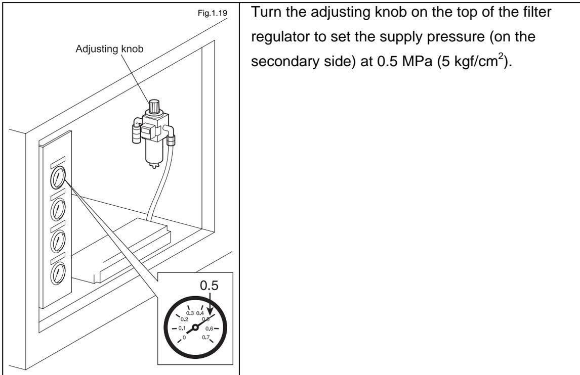
The supply pressure to each module is as specified below.
