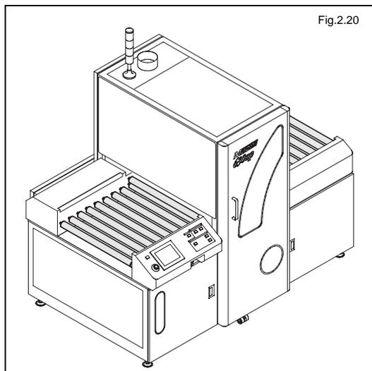
Laterally wipe any dirt off the conveyor rolls using a dust-free cloth moistened with methyl alcohol.
