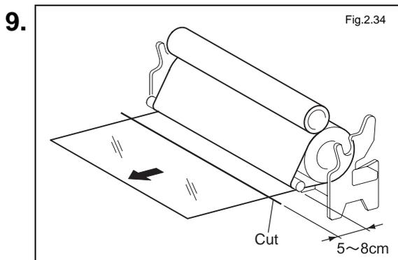
Cut the laminate film leaving a section 5 cm to 8 cm in length extending from the cover-film separation roll.
