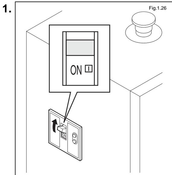
Supply power to the primary side of the plant and turn on the main breaker ON (I). The main breaker is located on the control box at the rear of the unit.
