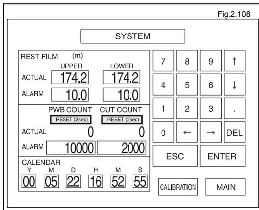
Hold down the "RESET" button for two seconds or longer.
