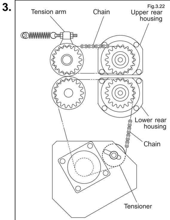
Before removing the rear housing, loosen and remove the roll-drive sprocket chain.
