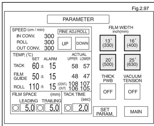
Select one of the four film widths that corresponds to the width of the loaded film.
