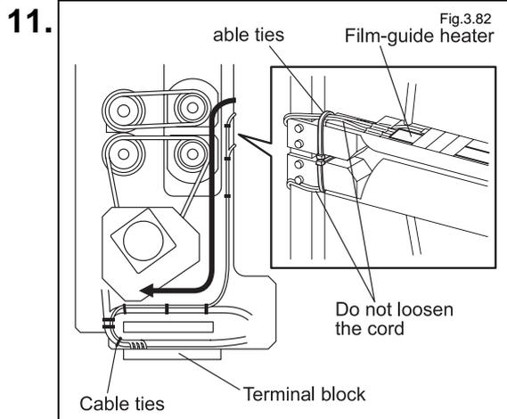
Use cable ties to fix the film-guide heater and sensor wires at the positions at which the removed cable ties were used, and connect the wires to the terminal block.
