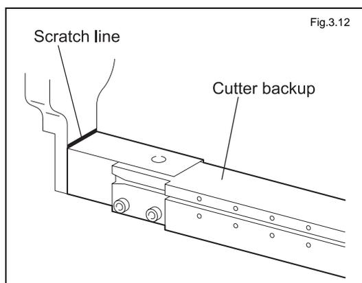
Before removing the cutter backup, scratch a line on the chassis to indicate the re-assembly position.
