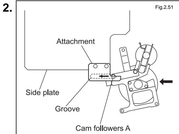
Place the front and rear cam followers A of the lower DF unit in the groove of the attachment. Lift cam followers B and insert the DF unit in the direction indicated by the arrow.
