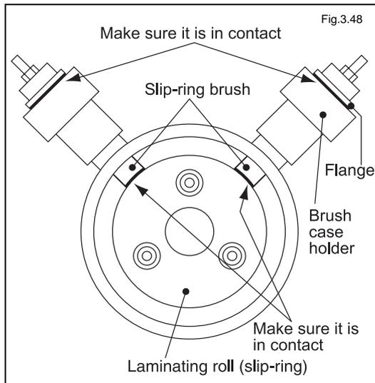
Fix the slip-ring cover and slip-ring-brush unit, and visually check the contact condition.
