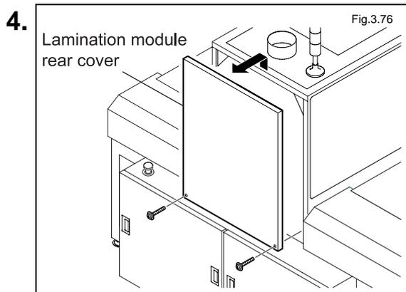
Remove the lamination module rear cover to provide access to the interior of the unit.
