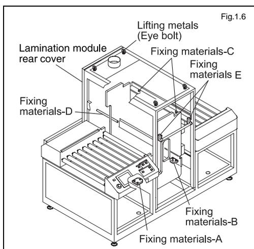
The fixing materials are used at the five locations on the unit shown in Figure 1.2.4 (left). Eye bolts for hauling are also fixed on the ceiling of the lamination module.
