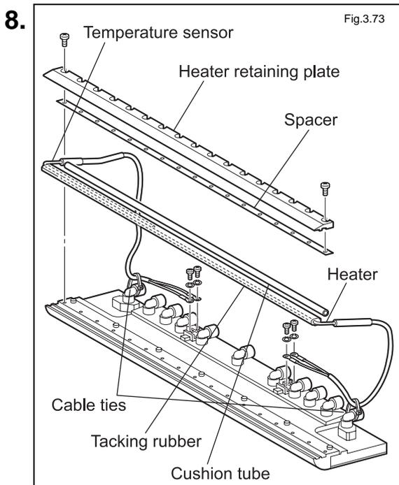
Remove the heater retaining plate, tacking heater terminal, tacking temperature-sensor terminal, tacking rubber, tacking heater, tacking sensor, and spacer.
