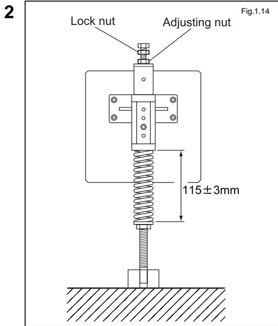
Adjust the tension of the pull-out casters.
