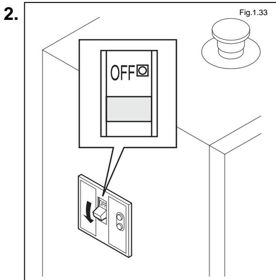
Turn off the main breaker OFF (O), which is on the control box at the rear of the unit.
