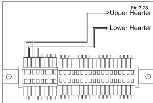
Remove the wires of the film-guide heater from the terminal block.
