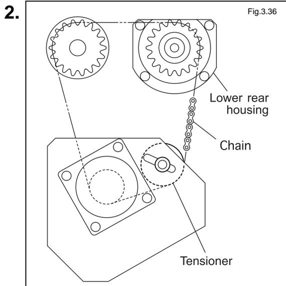
To change the tension of the lower rear housing-roll drive sprockets, adjust the tensioner after loosening the tensioner screw.
