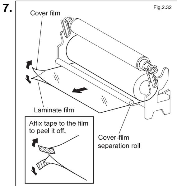
Pull out the dry film, and run it under the cover-film separation roll to separate the laminate film from the cover film.
