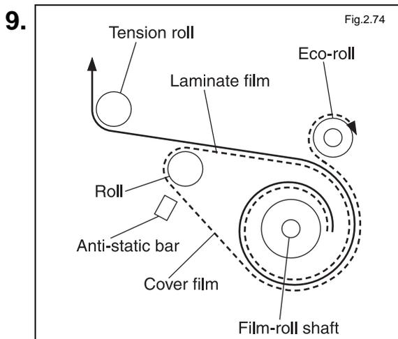
The dry film has now been loaded into the lower DF bulk unit, along the route shown in the illustration to the left.
