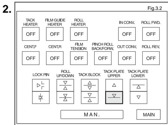
On the manual screen of the operation panel, press the TACK PLATE UPPER "CLOSE" button to move the upper tacking plate to the closed position.
