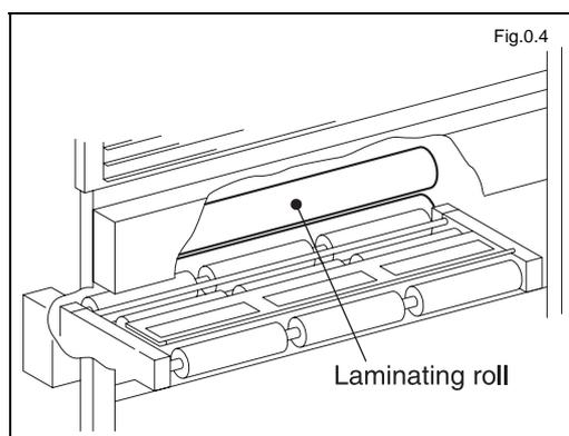
The lamination module of the unit has a laminating roll that rotates at high temperatures.
