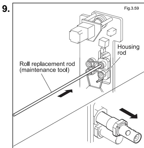
Screw the roll replacement rod (maintenance tool) into the laminating roll shaft, and push it toward the front of the unit.
