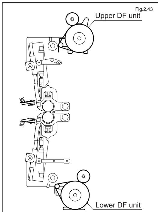
Place the upper and lower DF units at the positions of the lamination module shown in the illustration left, then run the laminate film to the lamination module.
