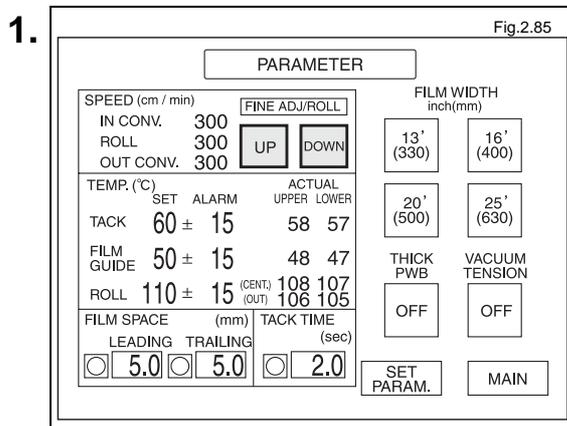
To increase or decrease the speeds of the input conveyor, output conveyor, and laminate roll, press the "UP" or "DOWN" button
