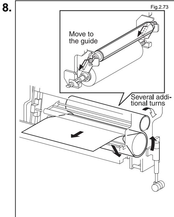
Fix the cover film to the eco-roll by running it under the dry film, and transfer the eco-roll from the holding groove to the guide section so it rests on the dry film.
