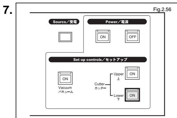
Press the Lower Cutter  button on the operation panel.
