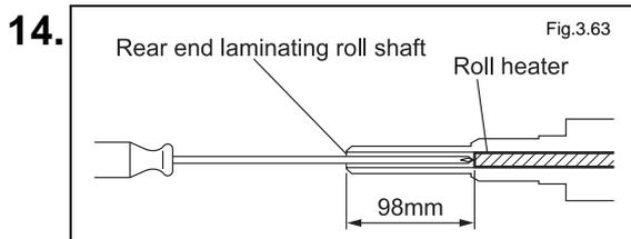
Insert a screwdriver into the rear end of the laminating roll shaft, and measure the current position of the roll heater.
