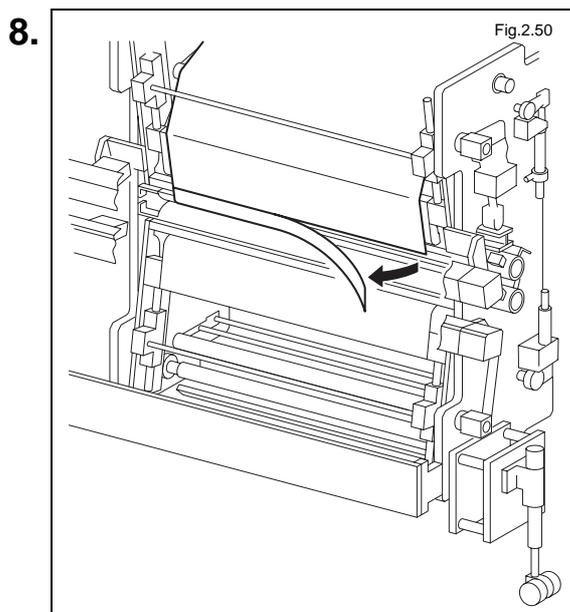
Remove the excess film that has been cut off.
