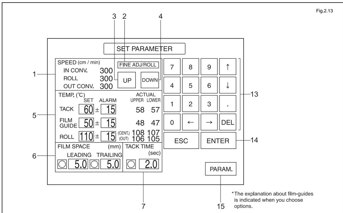
To return to the parameter screen, press the "PARAM." button on the parameter setting screen.
