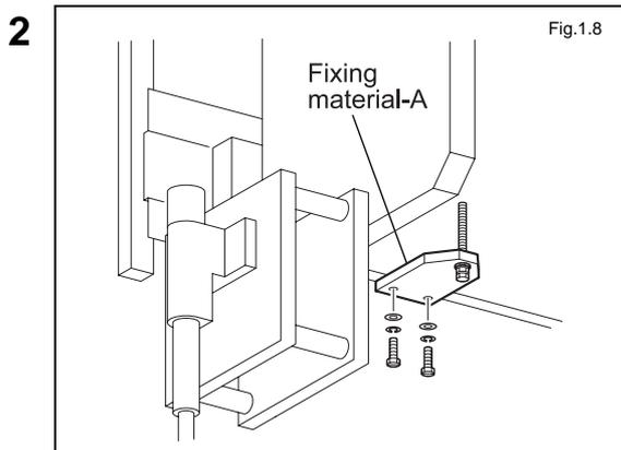
Remove fixing material A.
