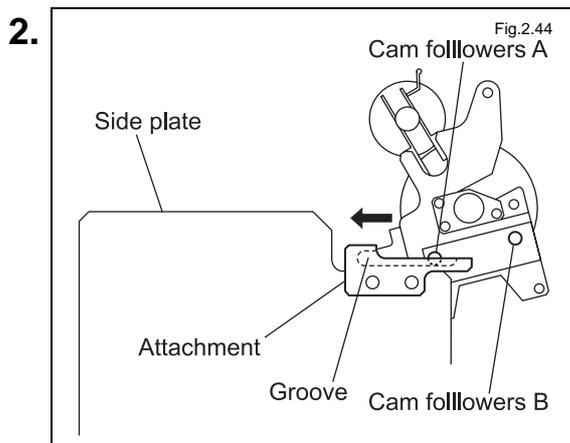
Place the front and rear cam followers A of the upper DF unit in the grooves of the attachment. Lift cam followers B and insert the DF unit in the direction indicated by the arrow.
