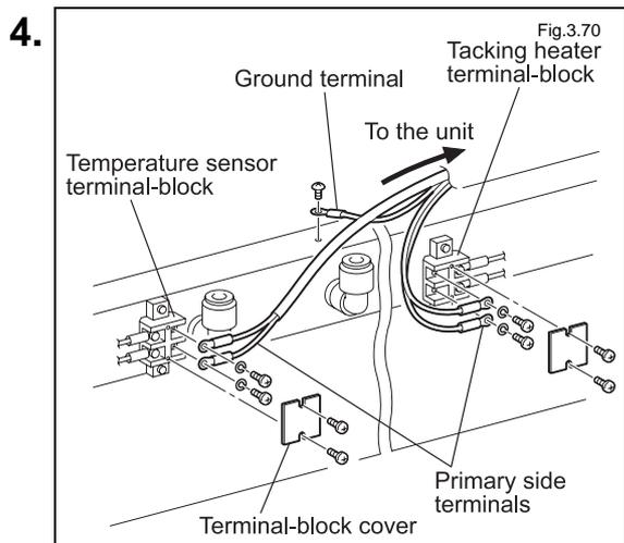
Remove the terminal-block covers and the primary-side terminals of the tacking heater and tacking temperature sensor. In addition, remove the GND terminal.
