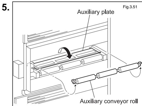
Open the auxiliary plate <sup>\*Option</sup> to remove the auxiliary conveyor roll.
