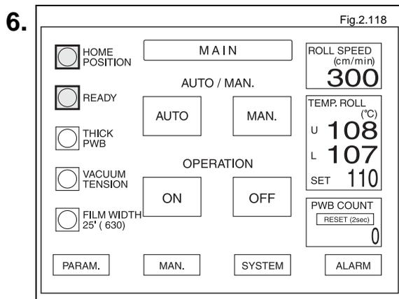
Return to the main screen and confirm that the "HOME POSITION" lamp and "READY" lamp are light. Press the OPERATION "ON" button to start automatic operation.
