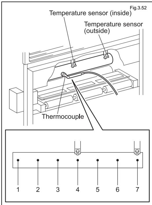
Press a thermocouple gently against the laminating roll to measure the surface temperature at the seven points specified below.
