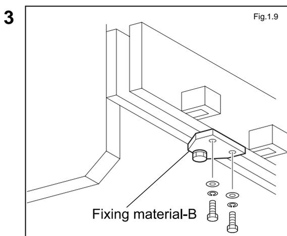
Remove fixing material B.
