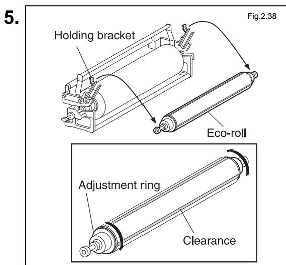
Remove the eco-roll from the DF unit and turn the adjustment ring to make a clearance on the external circumference.
