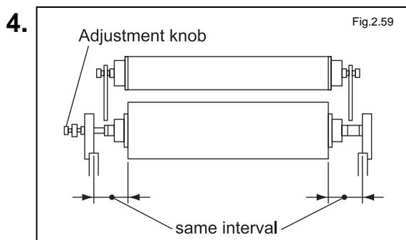
Place the film-roll shaft loaded with the dry film into the upper DF bulk unit.
