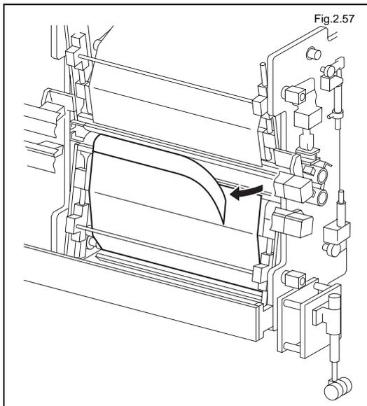
Remove the excess film that has been cut.
