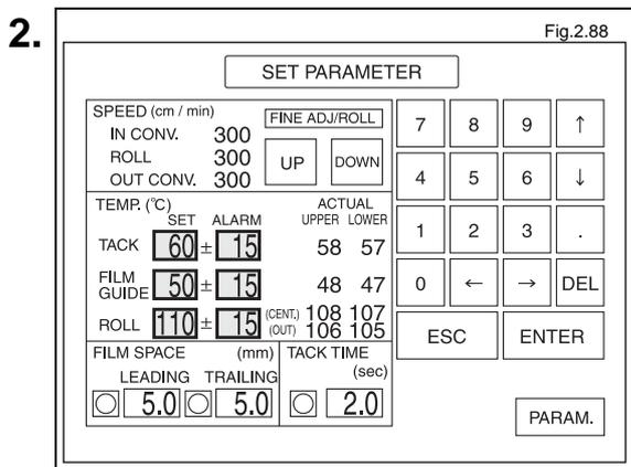
Press the square frame of the "SET" or "ALARM" temperature to be changed.
