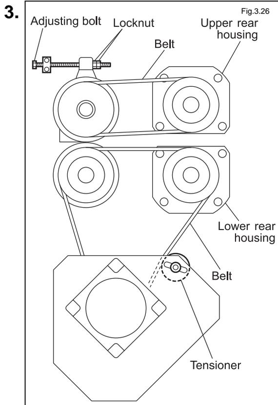
Before removing the rear housing, loosen and remove the roll-drive pulley belt.
