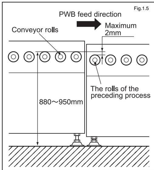
Adjust the height of conveyor rolls using the leveling feet. The height of the conveyor-roll surface from the floor must be between 880-mm and 950-mm.
