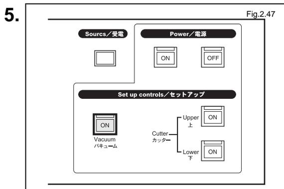
Run the laminate film down to the film guide and press the Vacuum  button on the operation panel.
