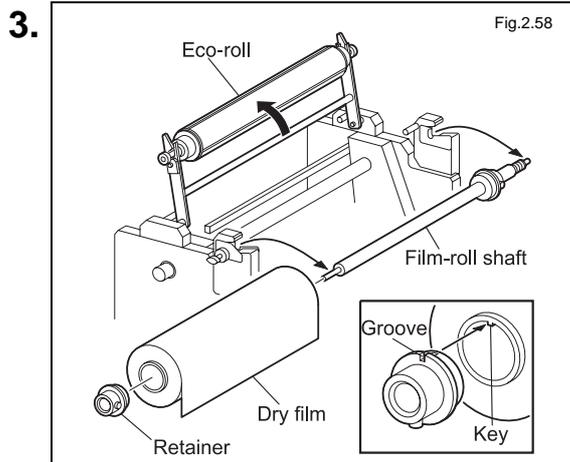
Lift the eco-roll of the upper DF bulk unit, remove the film-roll shaft and position the dry film at approximately the center of the shaft.
