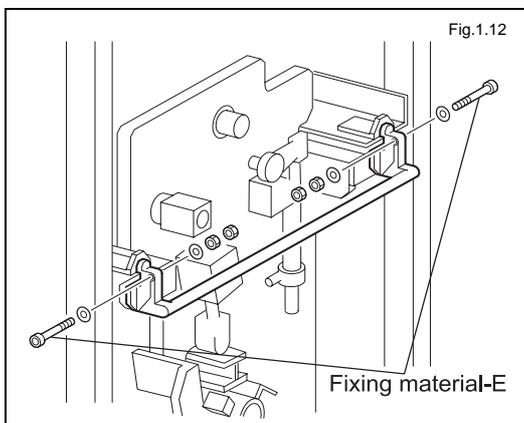
Remove fixing material E.
