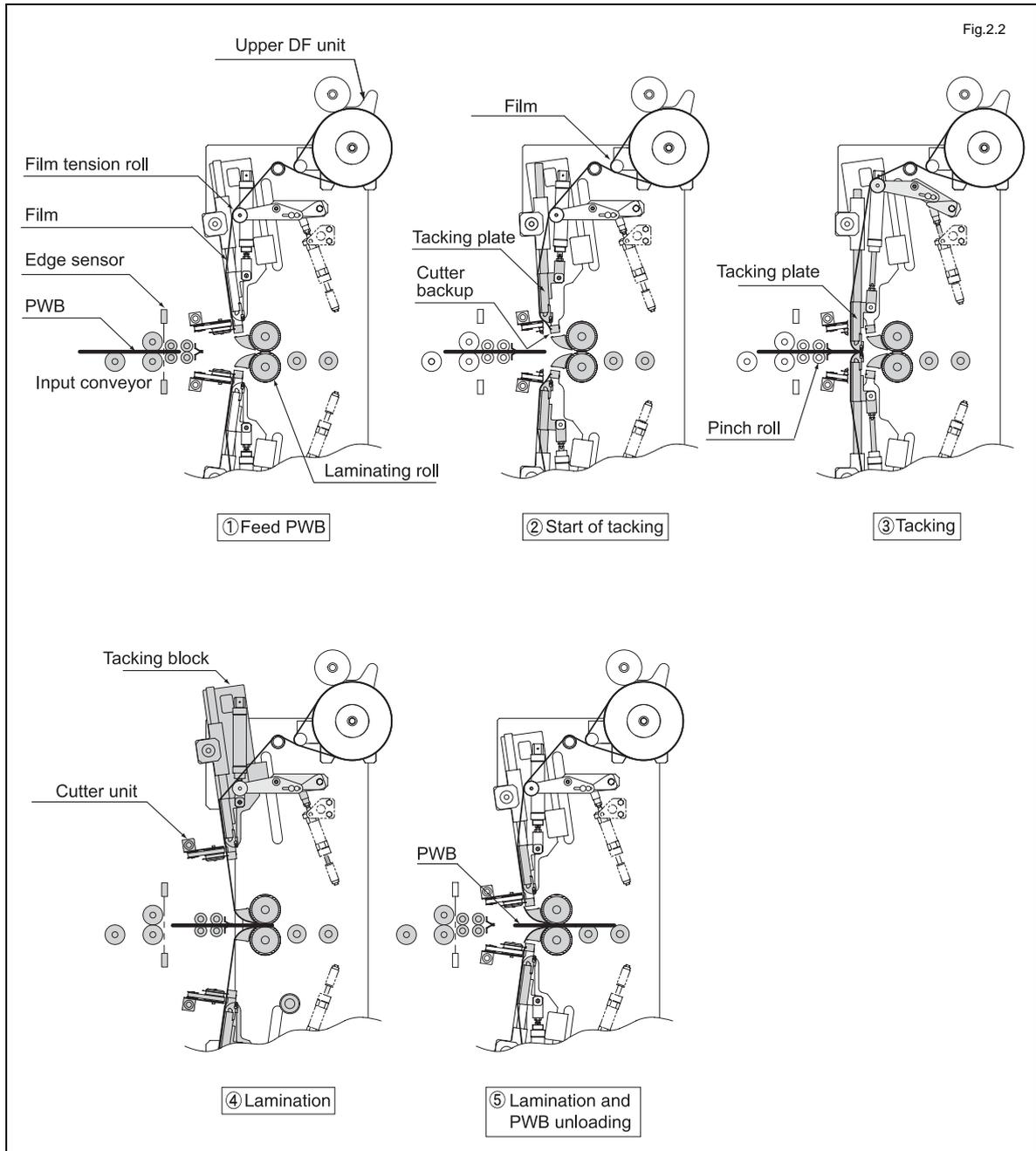
※ The above illustration shows the motion of the upper lamination module. The motion of the lower lamination module is symmetrical with that of the upper.
