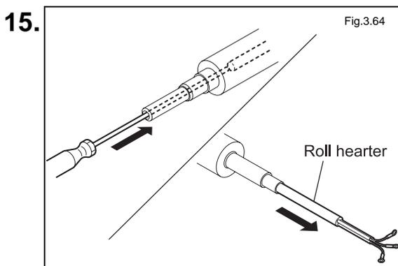
While wearing gloves, insert a screwdriver into the rear end of the laminating roll shaft. Push the roll heater with the screwdriver, and pull it out from the front end.
