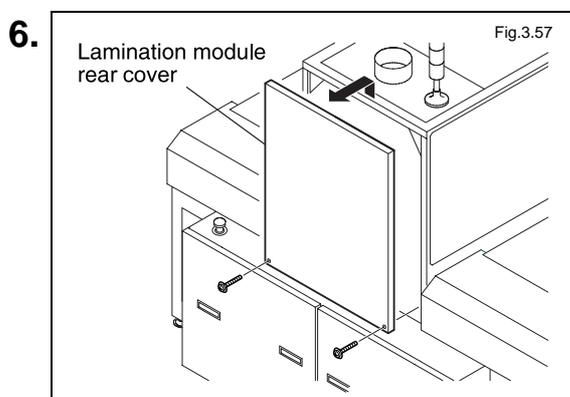
Remove the cover at the rear of the lamination module.
