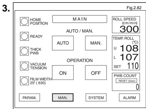
Press the white "MAN." button at the bottom of the main screen.
