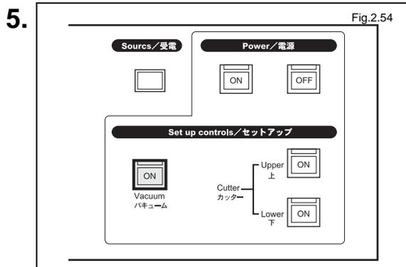
Run the laminate film up to the film guide, and press the Vacuum  button on the operation panel.
