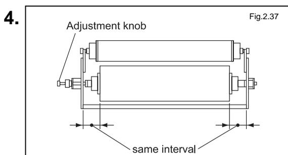
Place the film-roll shaft loaded with the dry film into the DF unit.
