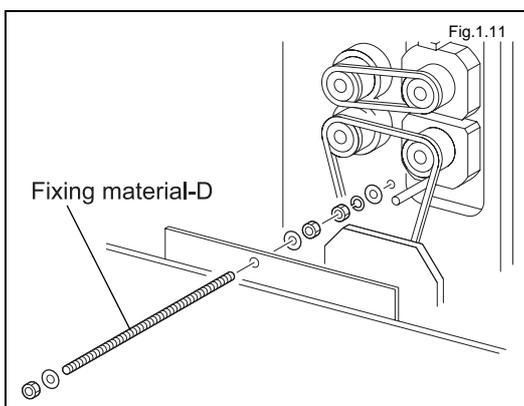
Remove fixing material D.
