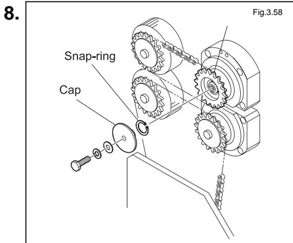
Remove the roll drive-pulley\* cap or the roll drive sprocket cap, and then remove the snap ring that attached to the roll shaft.
