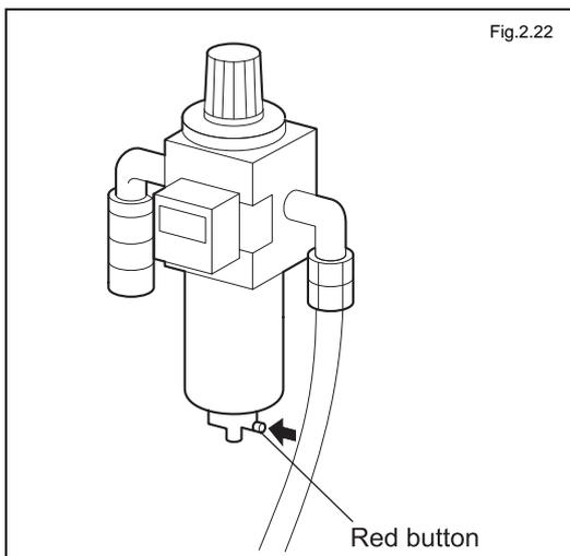
If there is any water or condensation in the filter bowl, press the red button at the bottom of filter bowl to drain it.
