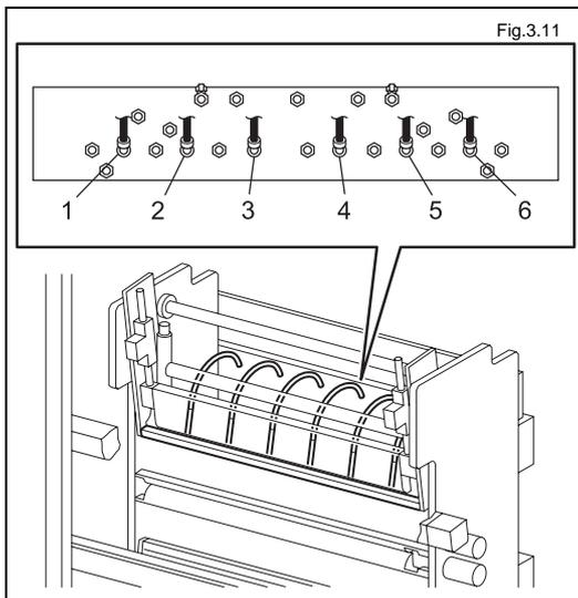
From the tube fitting at the innermost end of the lamination module, remove the six vacuum tubes extending from the cutter backup.
