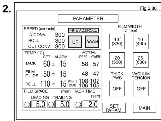
To finely adjust only the "ROLL" (laminating roll) speed, press the "UP" or "DOWN" button while holding down the "FINE ADJ/ROLL" button.
