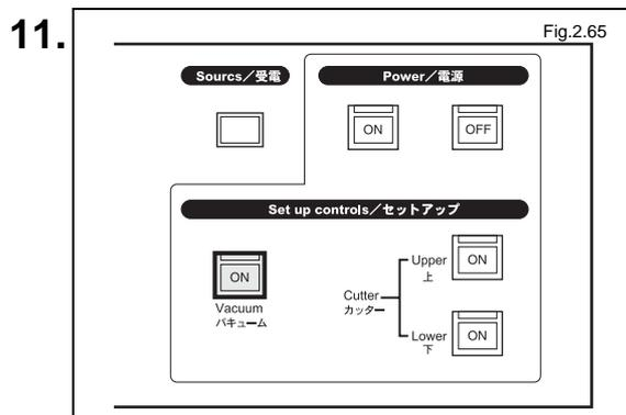
Run the laminate film down to the film guide and press the Vacuum [ON] button on the operation panel.
