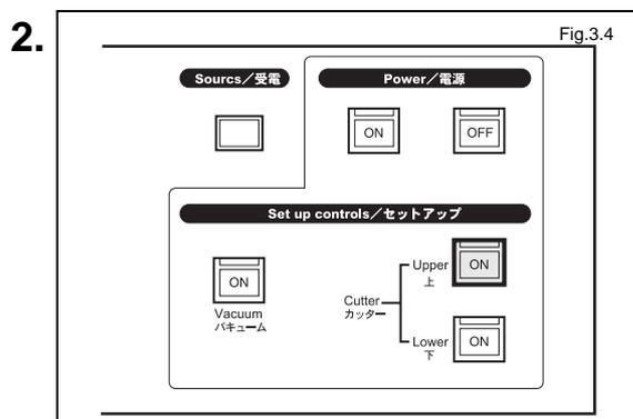
Press the Upper-Cutter  button on the operation panel to move the upper cutter assembly to the front side of the unit (if necessary).
