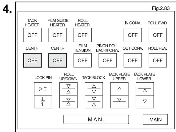
Press the CENT. F "OFF" and CENT. R "OFF" buttons to activate centering plates (F) and (R). Adjust the centering width to the width of PWB.
