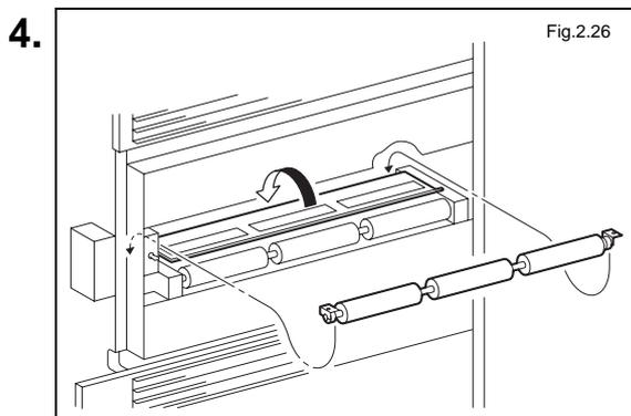
Upon completion of cleaning, fix the auxiliary conveyor roll and close the auxiliary plate <sup>\*Option</sup>.
