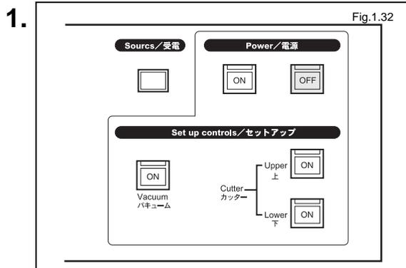
Open the cover of the Power  switch and press the button.
