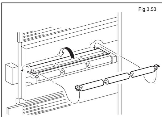
After measuring the temperature distribution, fix the auxiliary conveyor roll and close the auxiliary plate <sup>\*Option</sup>.
