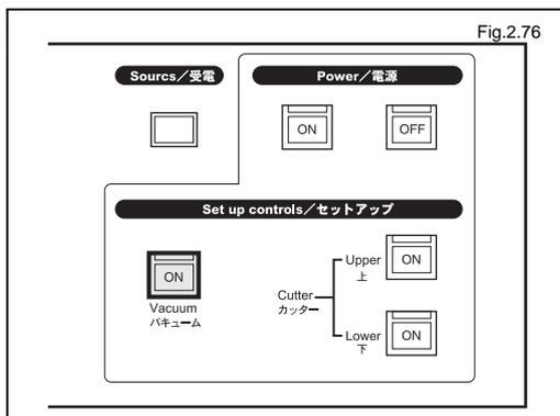
Run the laminate film down to the film guide and press the Vacuum  button on the operation panel.
