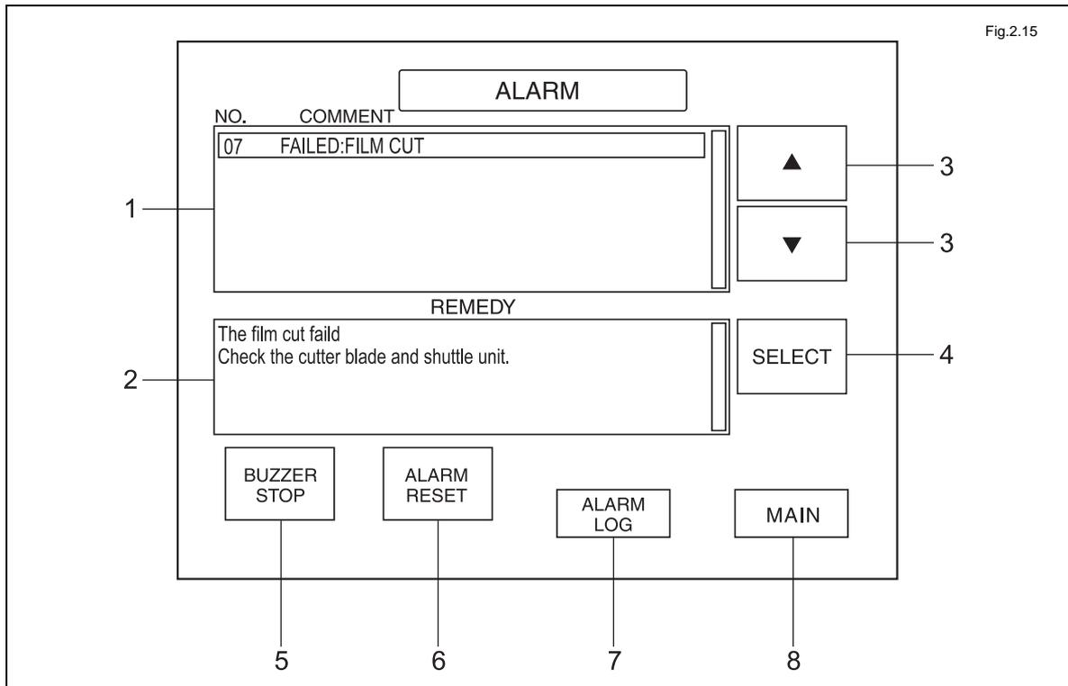
To switch to the alarm-log screen shown in the illustration below, press the "ALARM LOG" button on the alarm screen.
