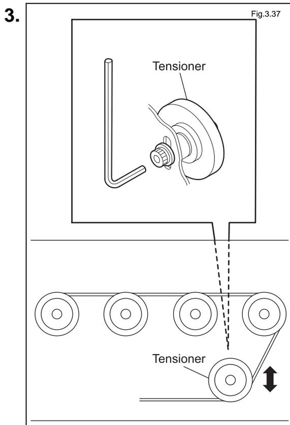
Adjustment of the Input/Output Conveyor Drive Chain
