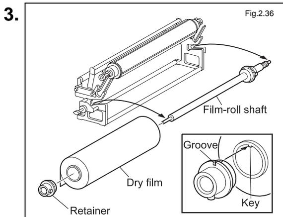
Remove the film-roll shaft from the DF unit and position the dry film at approximately the center of the shaft.
