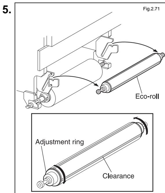
Remove the eco-roll from the lower DF bulk unit and turn the adjustment ring to make a clearance on the external circumference.
