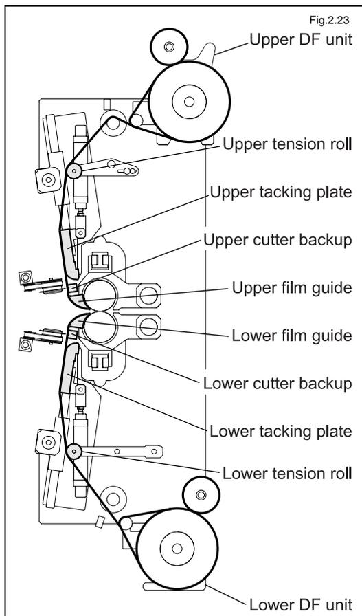
Wipe the film-running surface with a dust-free cloth moistened with methyl alcohol.
