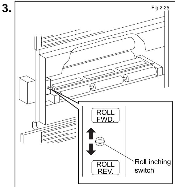
Turn the roll inching switch to "ROLL FWD." "ROLL REV." and laterally wipe away any dirt from the laminating roll surface and auxiliary conveyor roll using a dust-free cloth moistened with methyl alcohol.
