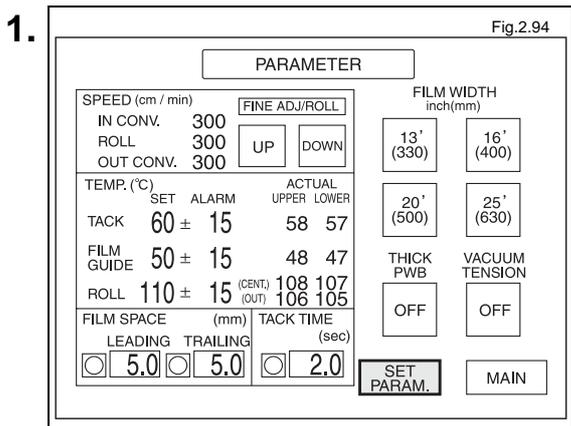
Press the "SET PARAM." button on the parameter screen to switch to the parameter-setting screen.
