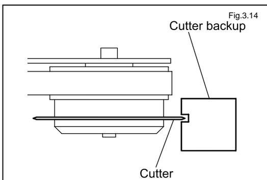
Carefully move the cutter assembly by hand back and forth in the cutter backup at low speed, to confirm that there is no interference between the two.
