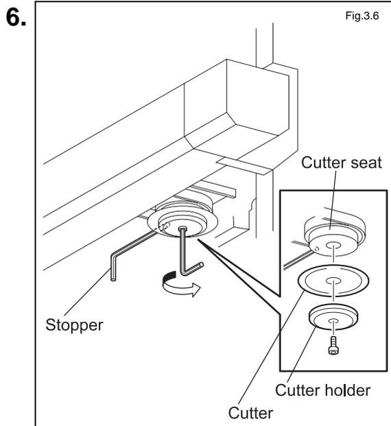
Remove the cutter and cutter holder.
