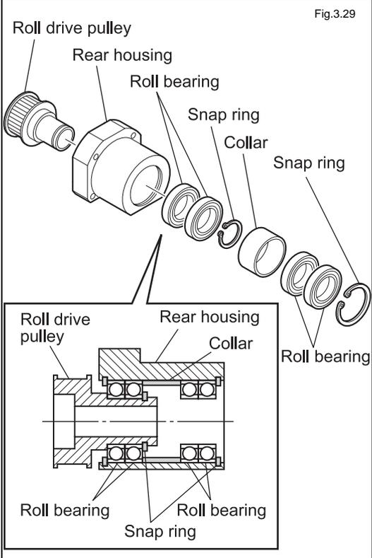
Remove the roll bearing of the rear housing. Remove the two snap rings. The roll bearing, collar, and roll drive pulley can now be pulled out.
