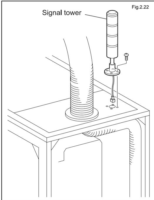
Fix the unpacked signal tower at the specified position on the ceiling of the lamination module.
