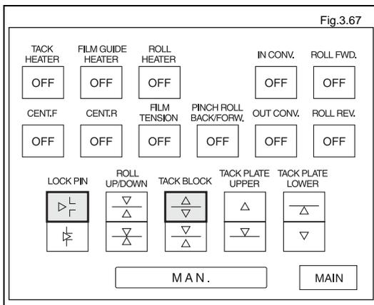
On the manual screen of the operation panel, press the LOCK PIN "RELEASE" button and TACK BLOCK "OPEN" button to move the tacking block to the open position.
