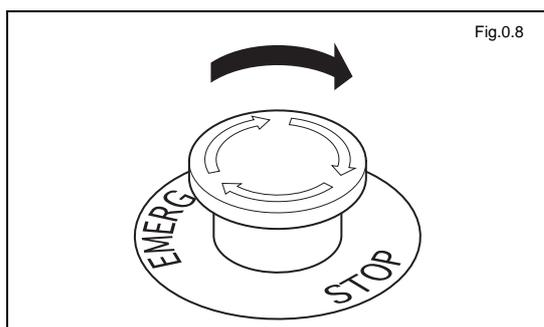
After correcting the problem, turn the button clockwise to release. Press the power  button on the operation panel to resume normal operation.
