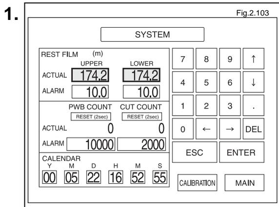
Press the square frame of the "ACTUAL" value of the REST FILM counter (m).
