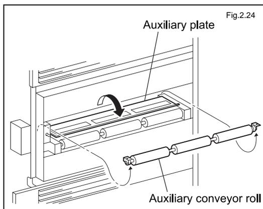
Open the auxiliary plate <sup>\*Option</sup> and remove the auxiliary conveyor roll.
