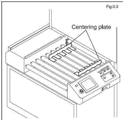
The input conveyor of the unit has a PWB centering mechanism that is driven by an air cylinder.
