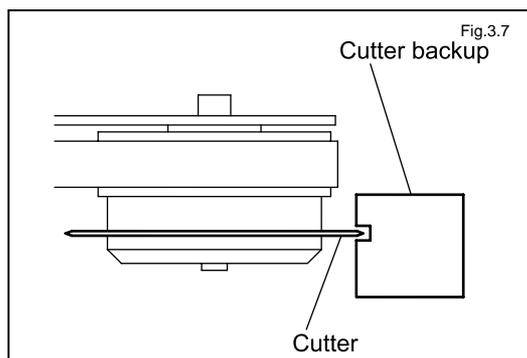
Manually move the cutter assembly back and forth slowly in the cutter backup to confirm that there is no interference between the two.
