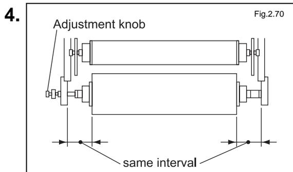
Place the film-roll shaft loaded with the dry film into the lower DF bulk unit.
