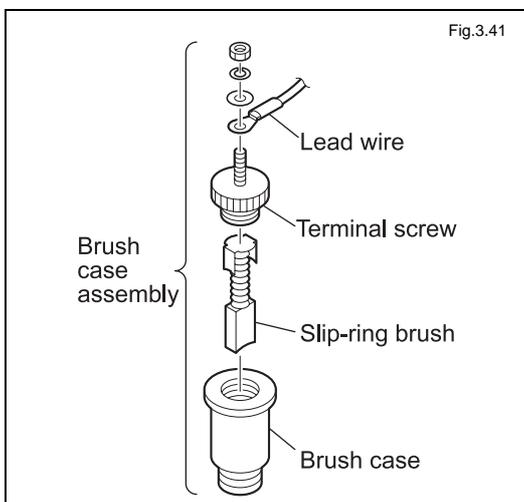
Remove the lead wires. Turn the terminal screws to remove the wires together with the brushes.
