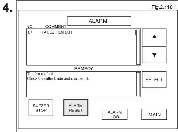
Press the "ALARM RESET" button to erase the alarm.
