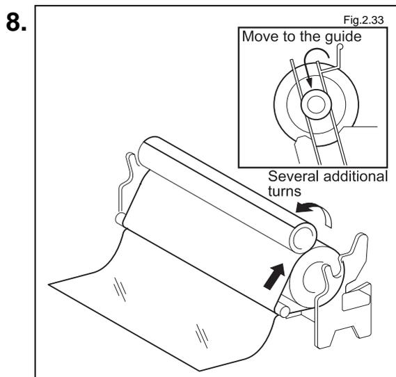
Fix the cover film to the eco-roll, and transfer the eco-roll from the holding bracket to the guide section. While separating it from the laminate film, wind the cover film several additional turns.
