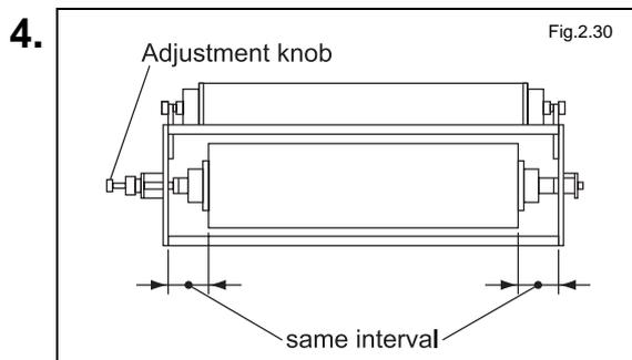
Place the film-roll shaft loaded with the dry film into the DF unit.
