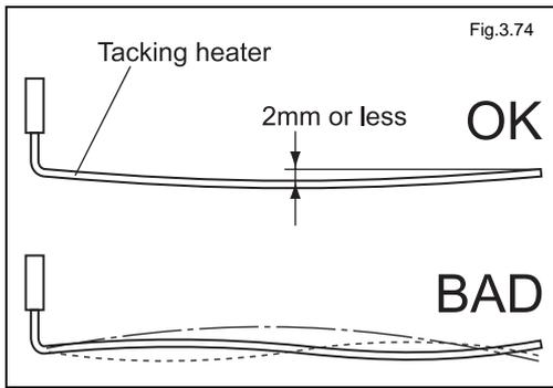
Do not bend the tacking heater or tacking temperature sensor.
