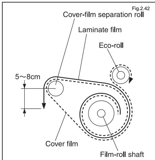
The dry film has now been loaded into the lower DF unit, along the route shown in the illustration to the left.
