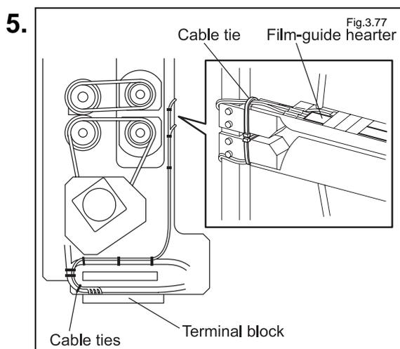
Cut the cable ties that fix the wires of the film-guide heater between the heater and the terminal block at the bottom of the lamination module.
