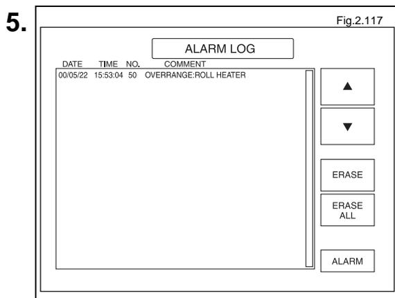
To display the log of past alarms, press the "ALARM LOG" button.
