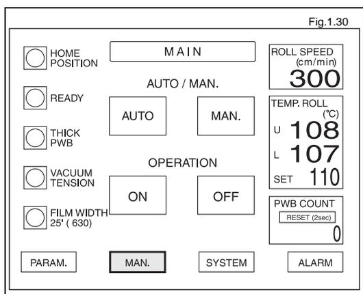
Press the white "MAN." button at the bottom of the main screen to access the manual screen.
