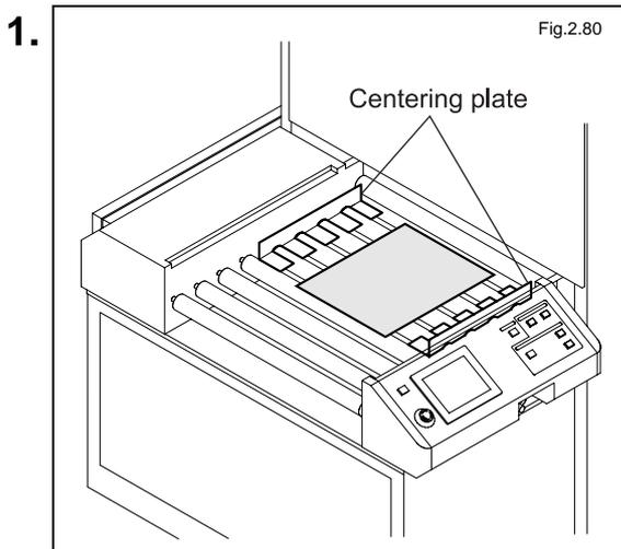
Place a PWB between the centering plates on the input conveyor.
