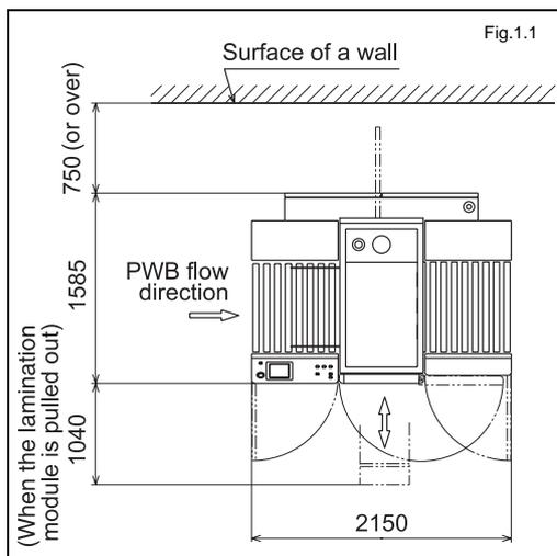
Secure an installation space, as shown in the illustration to the left, as well as space to move the unit safely to that installation space.
