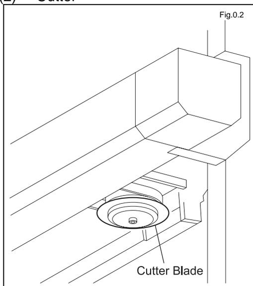
The unit has a rotary cutter for cutting films.
