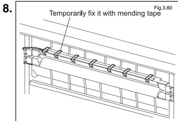
Apply adhesive uniformly to a new film-guide heater, and affix the heater to the film guide at the marking-off line. Temporarily fix the heater using scotch tape at several locations. Wait until it becomes completely bonded before removing tape.
