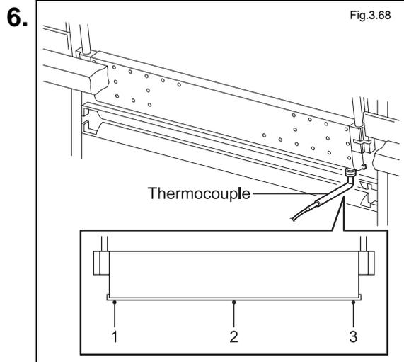
Press a thermocouple against the rubber at the tip of the tacking plate, and measure the surface temperature at the three points specified below.
