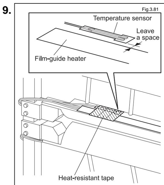
After the film-guide heater is completely bonded, remove the scotch tape temporarily holding the heater in place, and affix the temperature sensor using heat-resistant tape.
