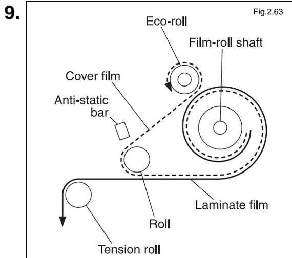
The dry film has now been loaded into the upper DF bulk unit, along the route shown in the illustration to the left.
