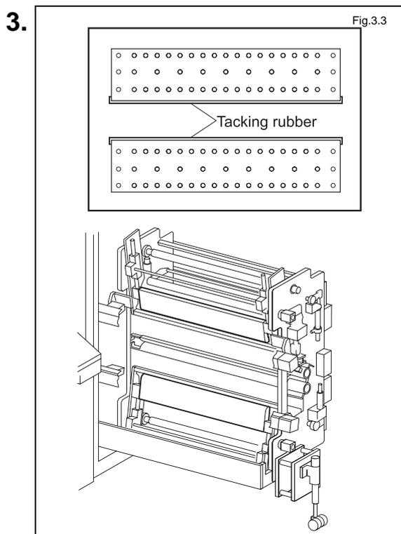
Wipe the tacking rubber in the lateral direction using a lint-free cloth moistened with methyl alcohol.
