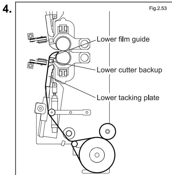
Run the laminate film along the film-running surface as shown in the illustration to the left.
