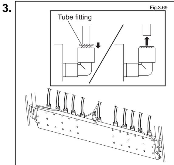
Remove the 11 air tubes attached to the tacking plate at the tube fitting.
