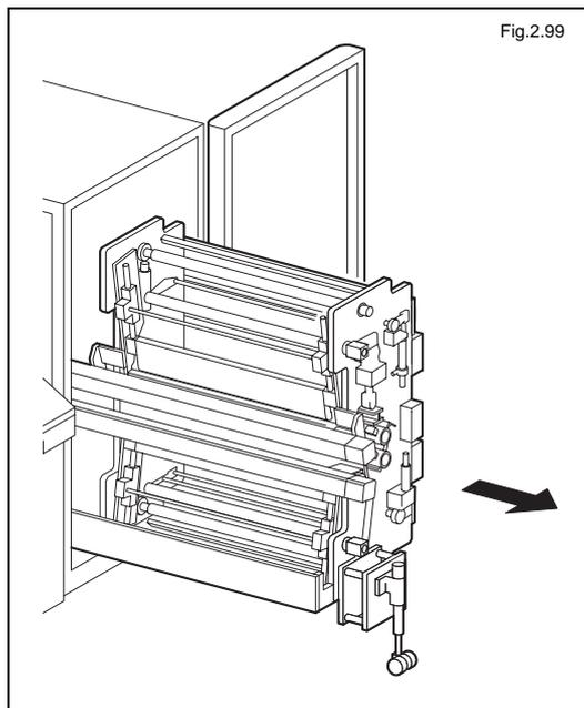
Open the front door and pull out the lamination module.
