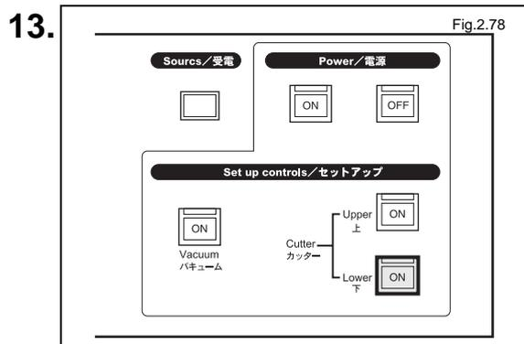
Press the Upper Cutter [ON] button on the operation panel.
