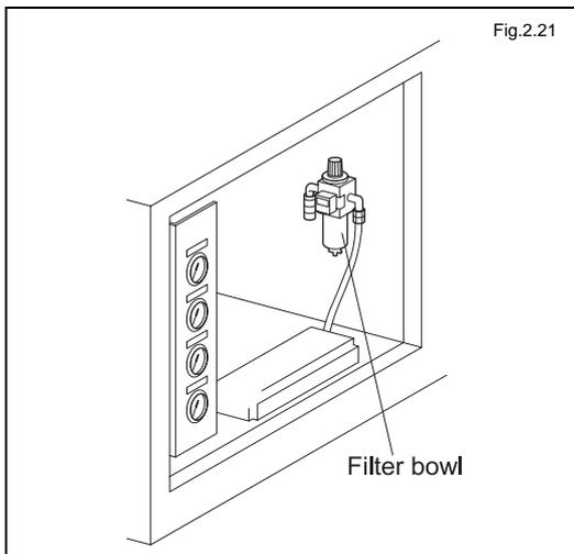
Confirm that there is no water or condensation in the filter bowl of the filter regulator unit.
