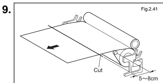
Cut the laminate film leaving a section 5 cm to 8 cm in length extending from the cover-film separation roll.
