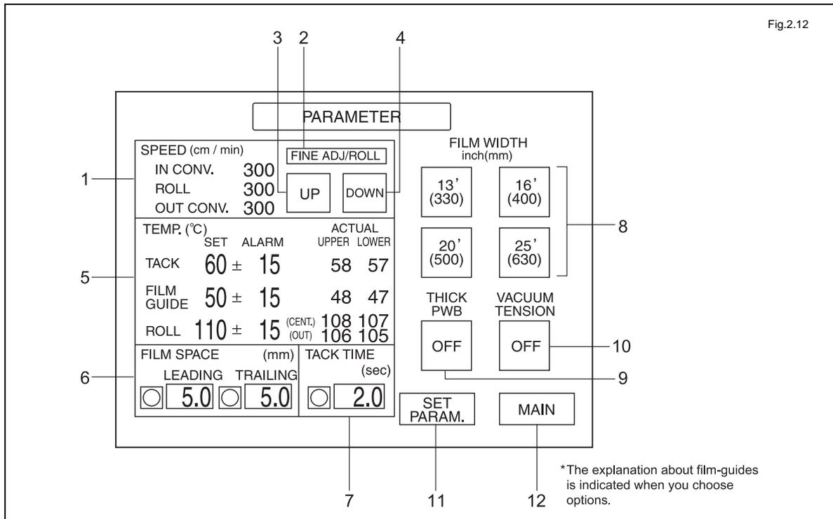
To switch to the parameter setting screen shown in the illustration below, press the "SET PARAM." button on the parameter screen.
