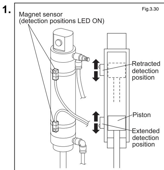
Loosen the screw of the band securing the magnet sensor, and align it with the piston by finding the ideal detection position (LED ON) when the piston is located at each end of the cylinder.
