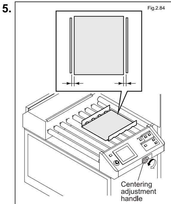
Turn the centering adjustment handle to set the distance between the centering plates to a value slightly greater than the width of PWB.
