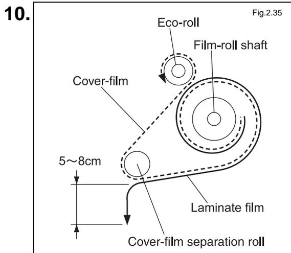
The dry film has now been loaded into the upper DF unit, along the route shown in the illustration to the left.
