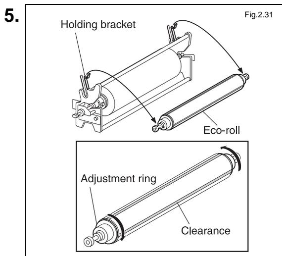
Remove the eco-roll from the DF unit and turn the adjustment ring to make a clearance on the external circumference. Making a clearance with the adjustment ring expands the diameter of the eco-roll slightly.
