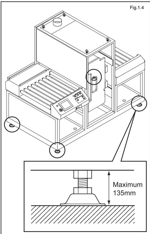
Fig.1.4 Adjust the height of the leveling feet at four corners.
