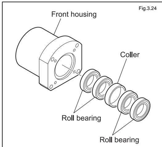
Remove the roll bearing of the front housing.
