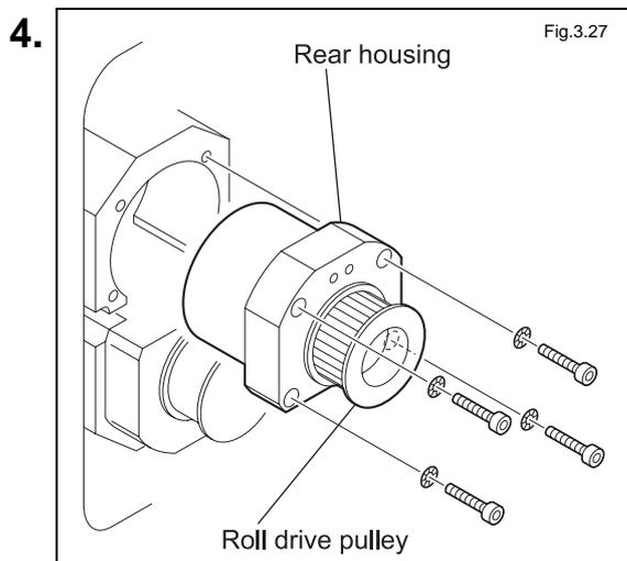
Remove the rear housing together with the roll drive pulley.
