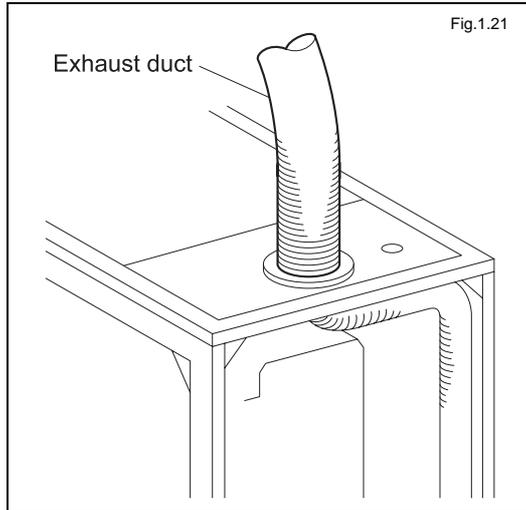
Confirm that the exhaust duct of the plant is connected to the exhaust duct on the ceiling of the lamination module.
