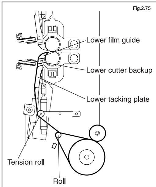
Run the laminate film along the film-running surface as shown in the illustration to the left.
