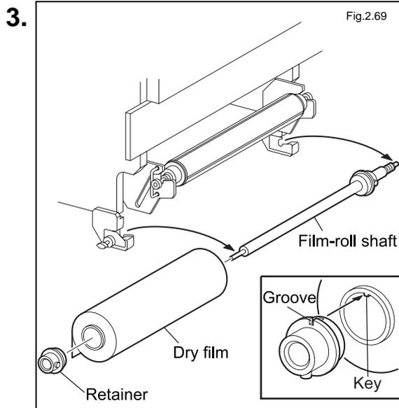
Remove the film-roll shaft from the lower DF bulk unit and position the dry film at approximately the center of the shaft.
