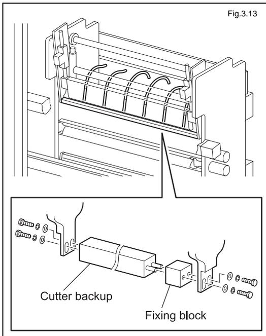
Remove the cutter backup by the method described below.
