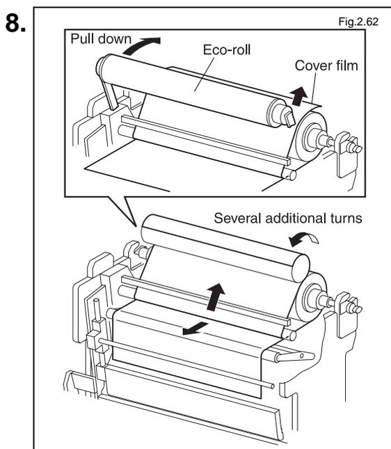
Fix the cover film to the eco-roll, and pull down the eco-roll so it rests on the dry film. While separating the laminate film from the cover film, wind the cover film several additional turns.
