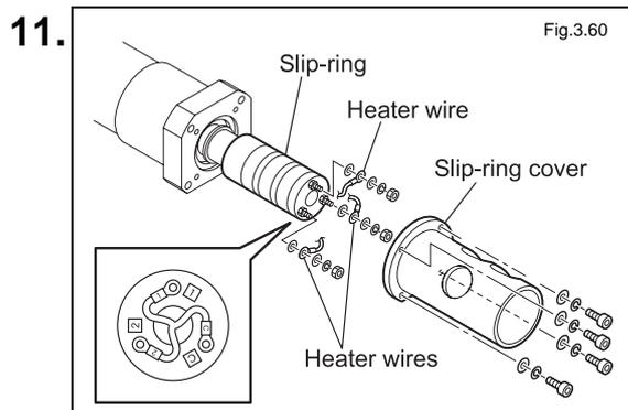
Remove the slip-ring cover and heater wires.
