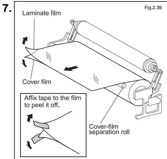
Pull out the dry film, and run it over the cover-film separation roll to separate the laminate film from the cover film.
