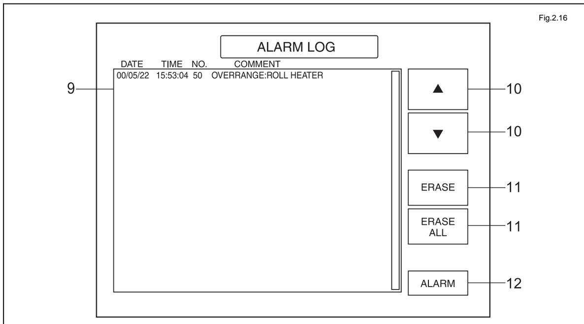
To return to the alarm screen, press the "ALARM" button on the alarm log screen.
