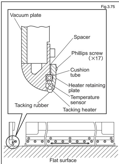
To assemble the tacking plate, temporarily assemble the components and place the assembled components upright on a clean, flat surface. Individually tighten the Phillips screws of the heater retaining plate, from the center toward the outside. See the illustration (left) for more information.
