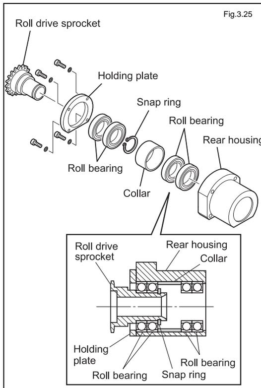
Remove the roll bearing of the rear housing.
