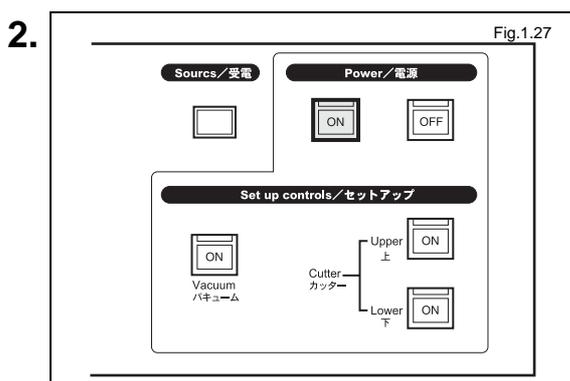
Open the cover of the Power **ON** button, and press the button.
