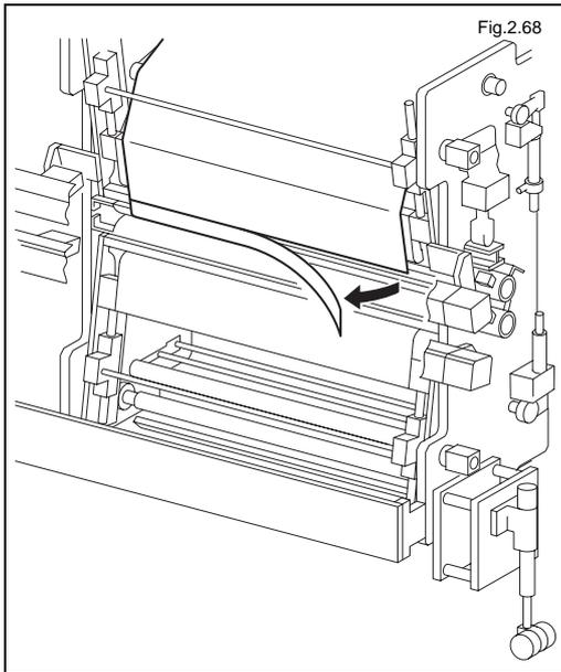
Remove the excess film that has been cut off.
