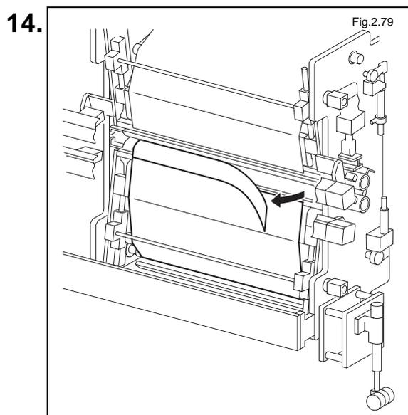
Remove the excess film that has been cut off.
