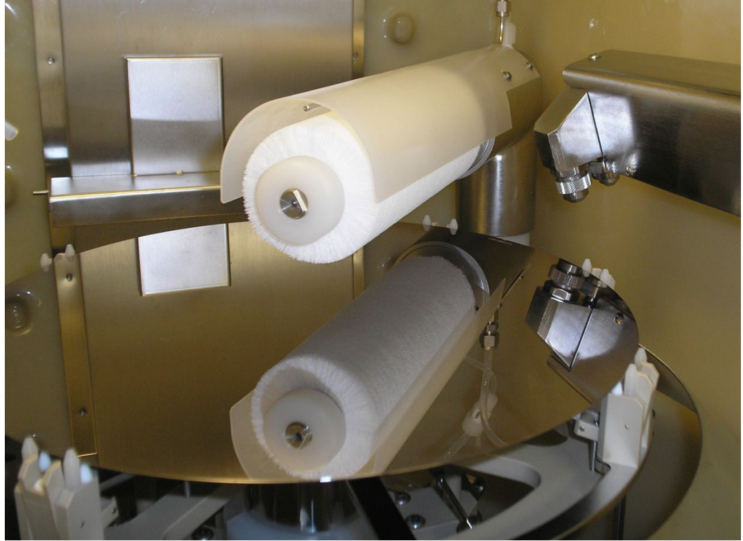
The Arm has swung out over the center of the wafer.
