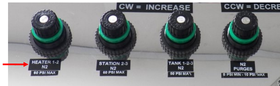
Figure 58 Regulator panel showing a Heater N2 knob (may also be labeled Dispense N2 )
