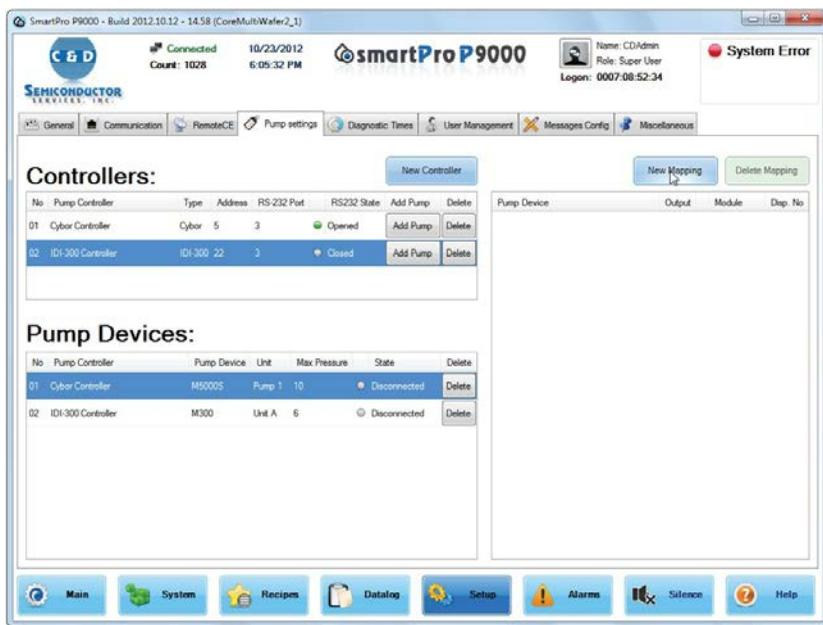
FIGURE 4-10: Mapping pumps with modules
