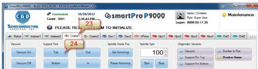
**FIGURE 6-9:** Centering the Coater
