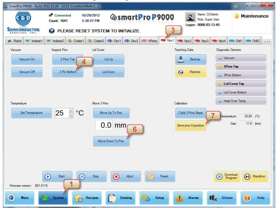
FIGURE 6-13: Calibrating height of support pins
