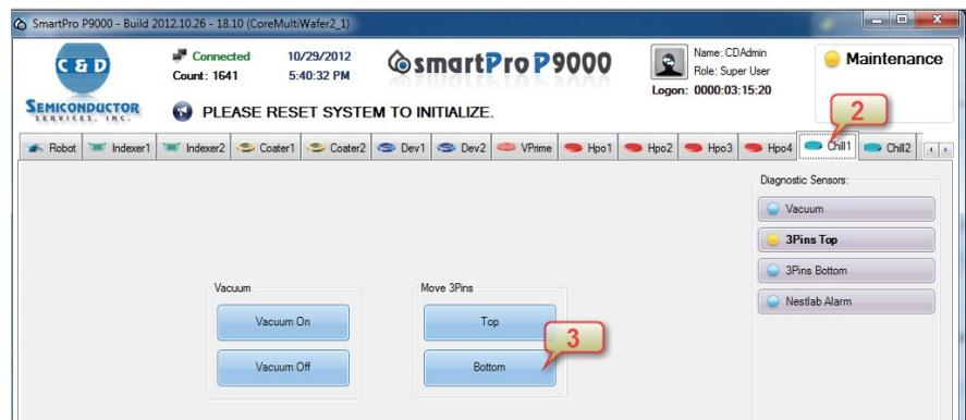
**FIGURE 6-10:** Centering the Chill Plate
