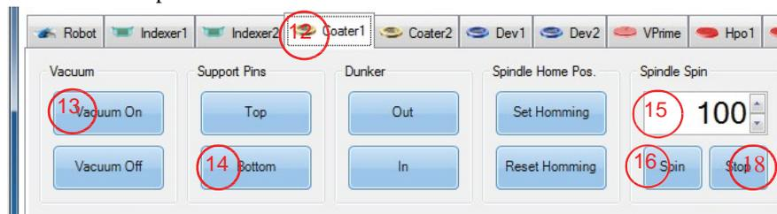
FIGURE 6-15: Checking Coater 1 low spin speed
