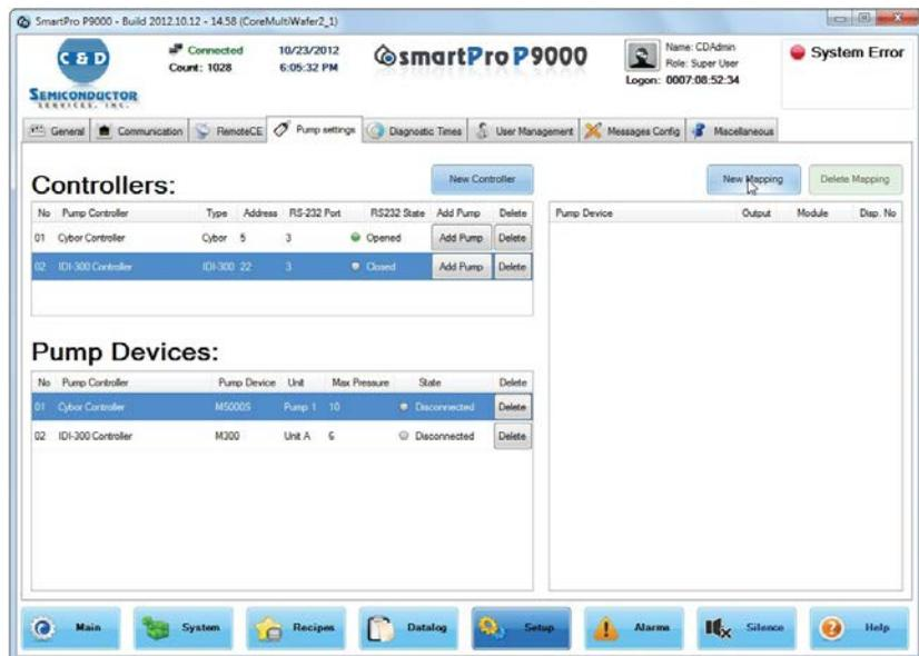
FIGURE 4-9: Pump settings page with sample pump controllers and pumps
