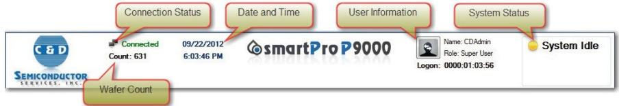
**FIGURE 1-2:** P9000 Operating Console Top Panel
