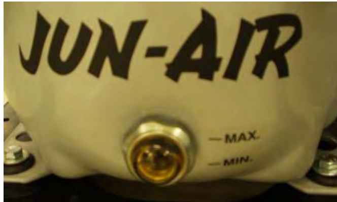
FIGURE 6-1 COMPRESSOR OIL LEVEL CHECK
